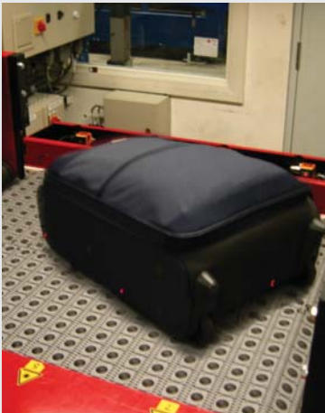
Eight PMD distance sensors are used to monitor the position of rotating luggage at Heathrow Airport. The sensor's red beam is visible on the suitcase above.
