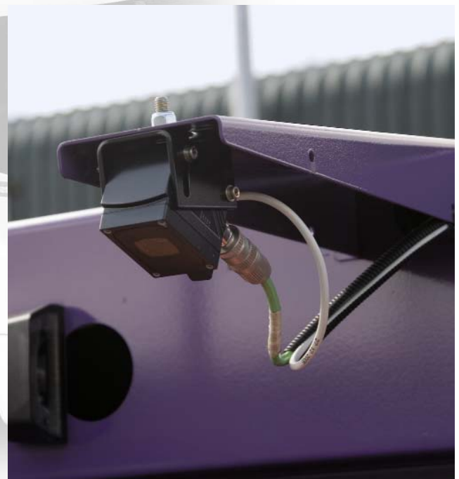
O2M Ethernet camera on a refuse truck
